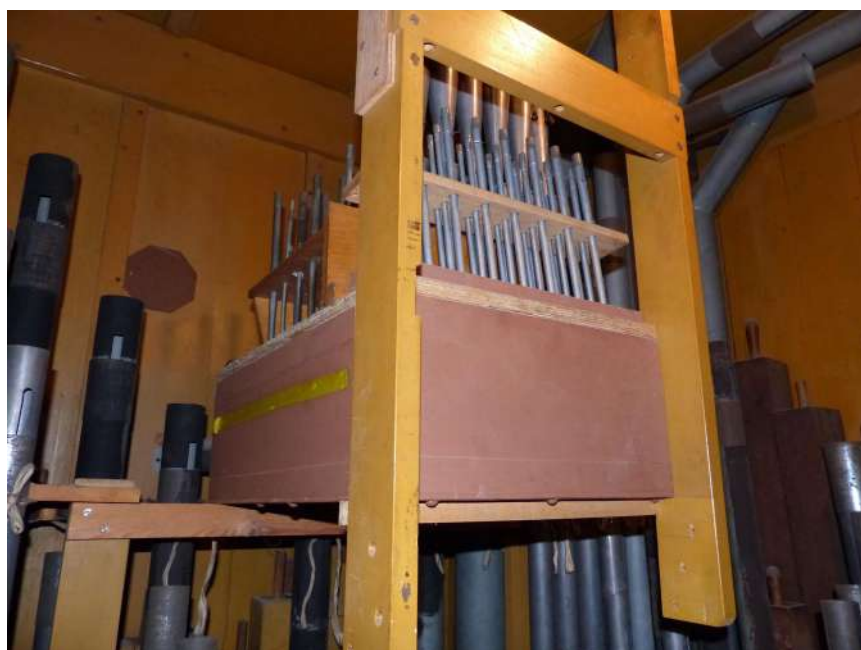
A 'top note machine' cluttering up the middle of the Swell box, severely hindering access for the tuner.
